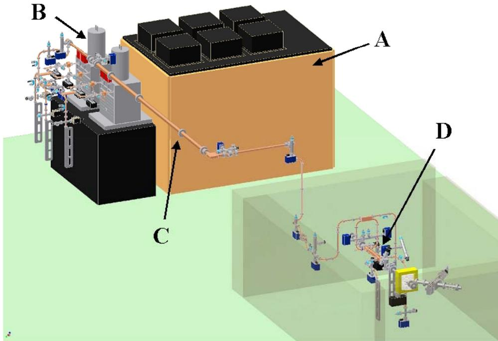
A: Modulator B: Klystrons C: Circular Waveguide D: Accelerator Structure in the Bunker. The control hut is not shown explicitly in the figure.
