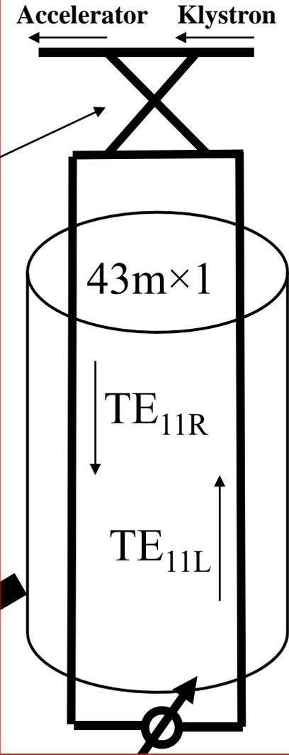
$$\begin{pmatrix} 0 \\ V(b2) \\ V(b3) \\ 0 \end{pmatrix} = \begin{pmatrix} 0 & \sqrt{1-k^2} & jk & 0 \\ \sqrt{1-k^2} & 0 & 0 & jk \\ jk & 0 & 0 & \sqrt{1-k^2} \\ 0 & jk & \sqrt{1-k^2} & 0 \end{pmatrix} \begin{pmatrix} V(a1) \\ 0 \\ 0 \\ V(a4) \end{pmatrix}$$
